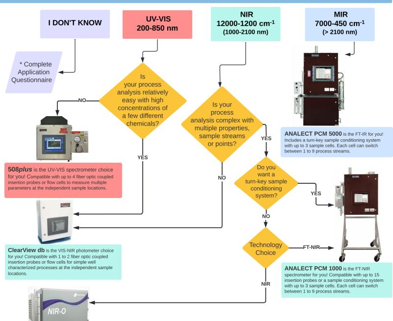
NIR-O is the Dispersive NIR spectrometer for you! Compatible with up to 12 fiber optic coupled insertion probes or flow cells to measure multiple parameters at the independent sample locations.
